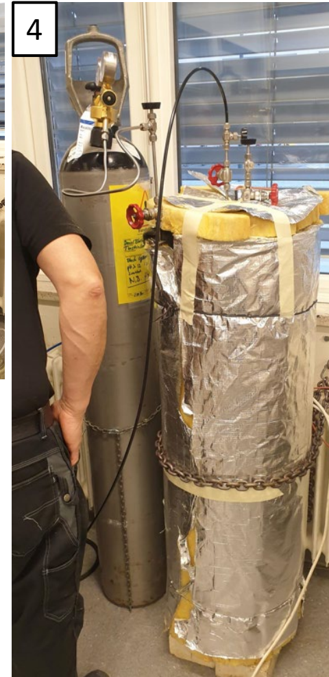
4 Isolating the autoclave over the heating bands
