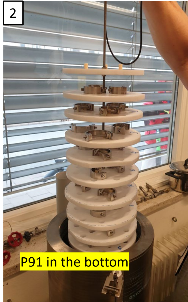
2 Inserting the samples to the autoclave and closing the lid
