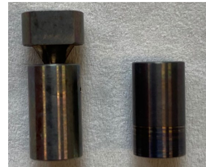
In-house made Titanium crucibles Grade 5
