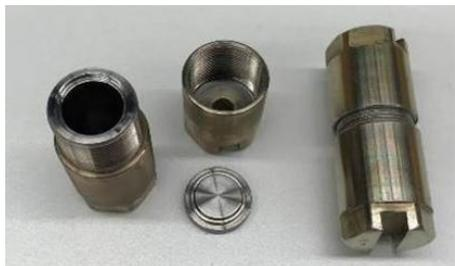
**Figure 2:** Micro autoclaves used for the batch experiments
