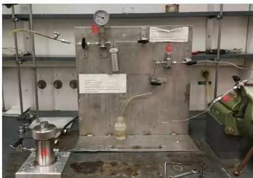
**Figure 3:** Micro autoclave station: a) Container for autoclaves; b) pressure measurement; c) septum for taking gas samples
