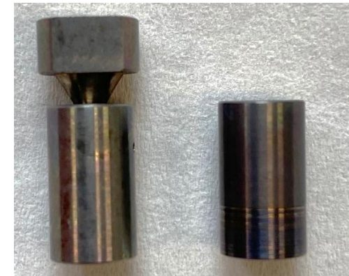
In-house made Titanium Grade 5 crucibles
